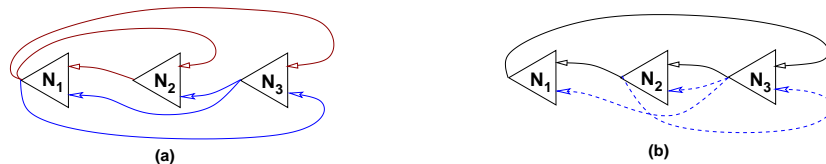
FIGURE 7. Three node identical cell system with nontrivial synchrony subspaces (a) (12), (123), and (b) (123).
