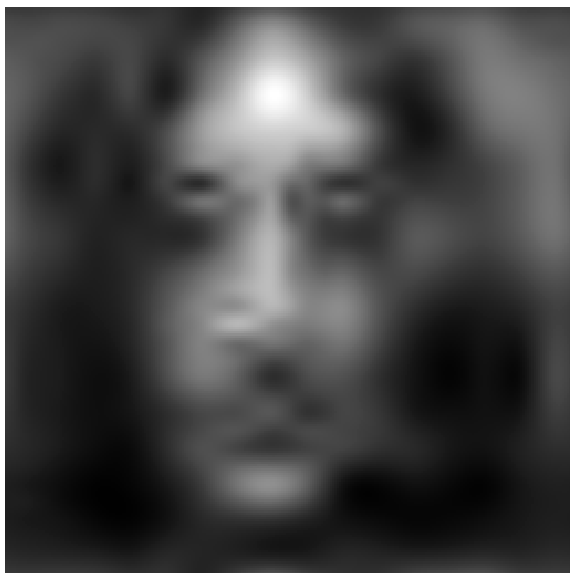
Figure 9: VisuShrink reconstruction of noisy image in Figure 8 using Daubechies' extremal phase wavelets N = 8 , soft thresholding and thresholding above level 3. The VisuShrink threshold was 534 and the integrated squared error between this reconstruction and the original was 6543.
