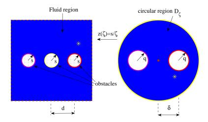
Figure 2: An example conformal map from a circular domain  $D_{\zeta}$  to the exterior of three circular obstacles.
