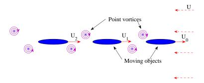
Figure 7: Three moving ellipse-like bodies in an ambient uniform flow together with an array of point vortices.
