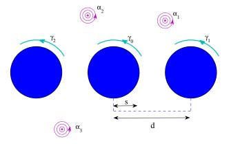
Figure 3: Three point vortices moving around three circular islands. There are non-zero circulations around each of the islands.
