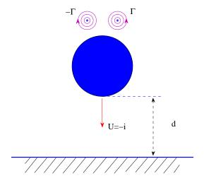
Figure 6: A moving cylinder, with point vortex wake, approaching a stationary wall at constant speed.
