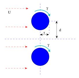
Figure 4: Uniform flow past two equal cylinders.
